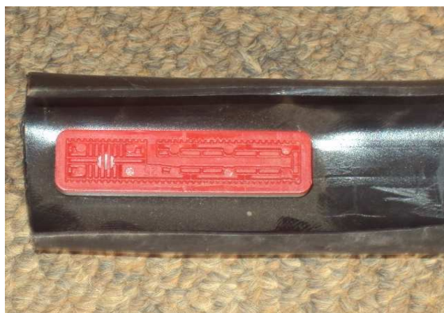
Figure 1: Cut section of a lateral showing pressure compensating in-line drippers
