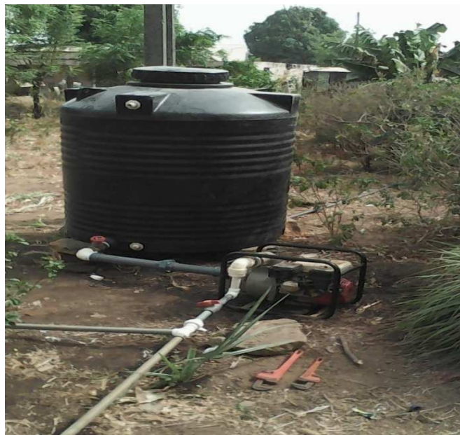
Figure 3: Gasoline pump delivering water from reservoir to the irrigation area
