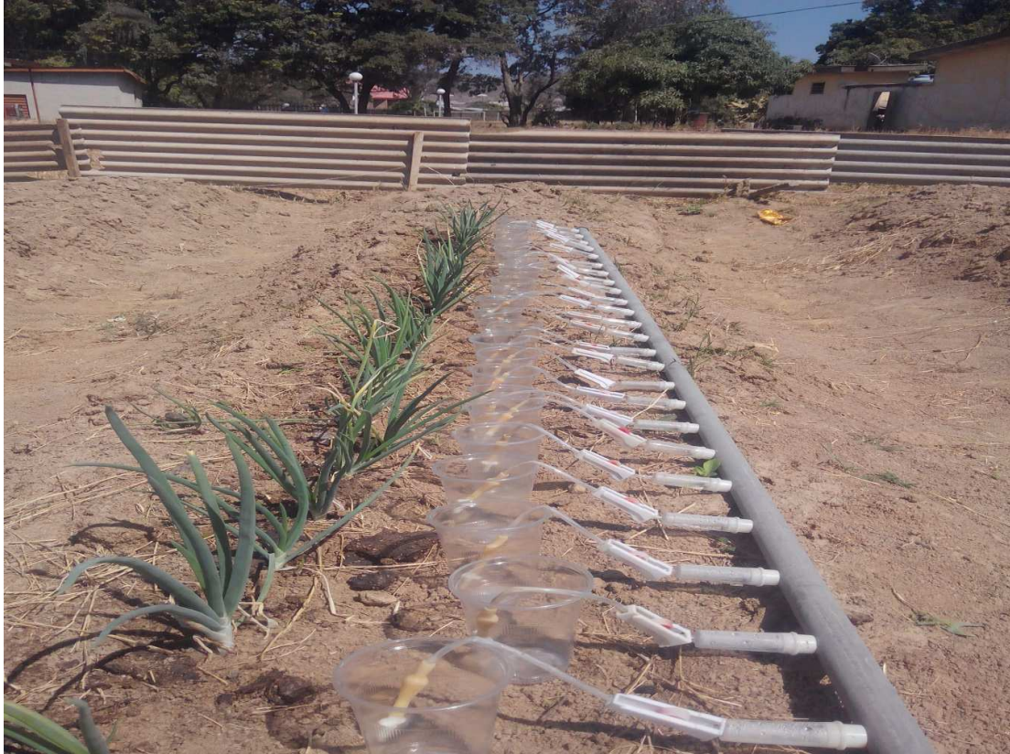
Plate 3: Catch can test for one of the junctions
