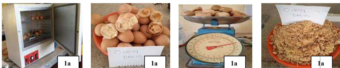
T3: Plates 1a, b, c and d: Boiled, oven dried and crushed fowl eggs
